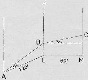
The diagram above represents part of the inside of two of the walls (built vertically and at right angles) of a parking station. In this diagram ALM represents the (horizontal) ground floor, and the lines AB and BC represent the ramp climbing up the two walls at a constant angle  $\alpha$ , where tan  $\alpha = \frac{1}{6}$ .
